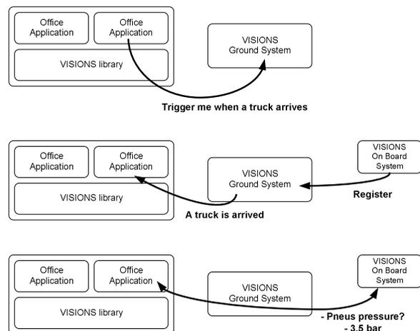
Fig. 2. VISIONS interaction scheme. Application interested in monitoring truck must register such interest on the VISIONS Ground System using VISIONS library. When a truck arrives in the covering area of a VISIONS ground system it registers itself on the Ground System and the Ground System triggers the interested applications. Finally, the application can query the On Board system for information.
