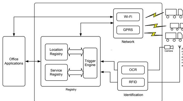
Fig. 3. The VISIONS Ground System architecture. VISIONS ground system is composed by three main blocks: the Registry, the Identification block and the Network block.
