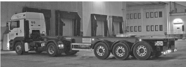
Fig. 7. VISIONS test vehicle. The commercial vehicle used for VISIONS experiments consists of a new generation tractor attached to an electronically equipped semi-trailer.
