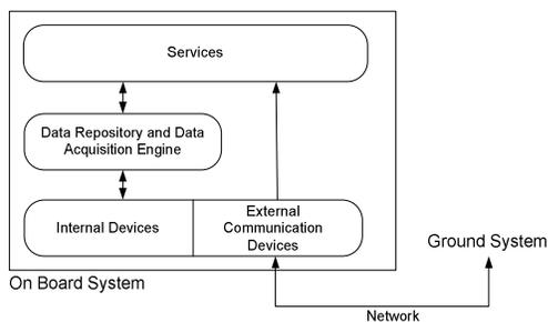
Fig. 6. VISIONS On Board System architecture.
