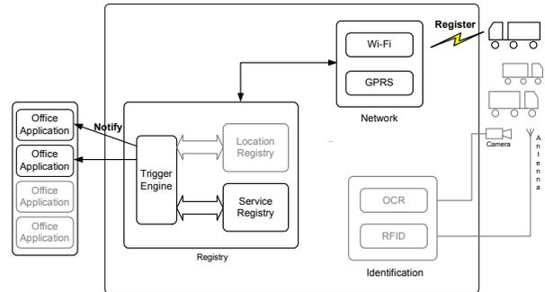
Fig. 4. Log on process. When a truck arrives in the covering range of the Ground system it registers itself on the Service registry. Then, the Trigger Engine signals the event to interested applications.
