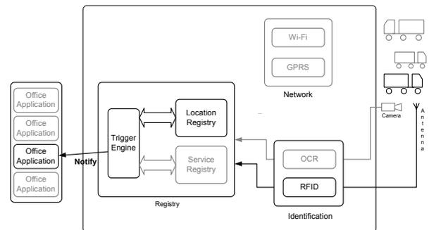
Fig. 5. Localization process. When a truck arrives at a point of interest, it is discovered by the RFID identification and the appropriate attribute is set on the Location Registry. Then the Trigger Engine signals the events to interested applications.
