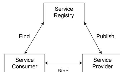
Fig. 1. Service Oriented Architecture basic interaction model. SOA defines three main actors: the Service Consumer, the Service Provider and the Service Registry. Providers publish the services they offer to a Service Registry. Consumers interrogate the Registry to discover the services they need and to obtain all the information needed to access such services.
