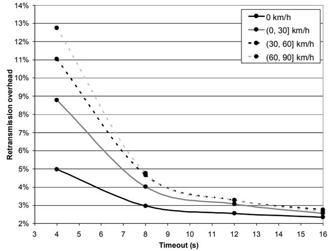
Fig. 6. Retransmission overhead  $\lambda$ . ( $L = 0.01$ )
