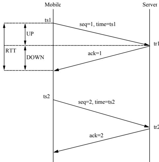
Fig. 1. Diagram of the stop-and-wait protocol adopted in the test system.
