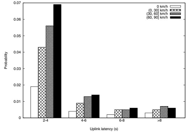
Fig. 4. Histogram ( $UP > 2$  s) of the uplink latency during the test period.
