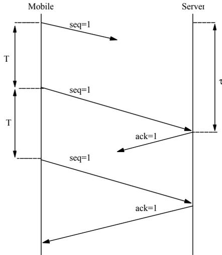
Fig. 5. Packet sequence diagram in case of an uplink loss during the first transmission followed by a downlink loss on the second transmission. In this case, there are two retransmissions and the message delivery time ( $\tau$ ) is the sum of the first timeout period ( $T$ ) plus the uplink time of the second transmission.
